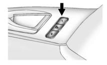
On vehicles with the memory package, memory buttons 1 and 2 on the driver door are used to save and recall memory settings for the driver seat cushion and seatback. outside mirrors, and the steering
